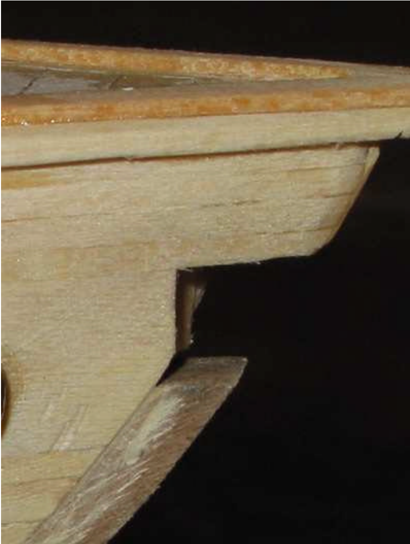
Photo 4: Bulwarks at bow. Note that they match the curve of the stem piece.
